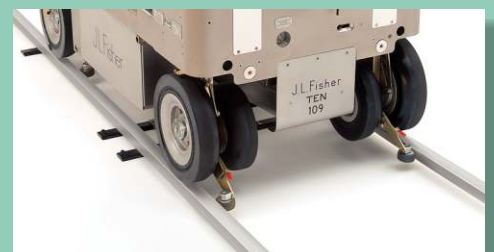
BUILT-IN TRACK GUIDES (Square Track Only)
